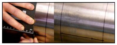
Figure 3-19: Measuring and Marking Spacing
